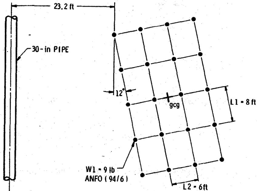
A 30-inch O. D. by 0.344 W. T. pipeline is adjacent to the grid as shown in the figure. The centerline of the pipe and the charges are 5 ft below the surface of the ground.
