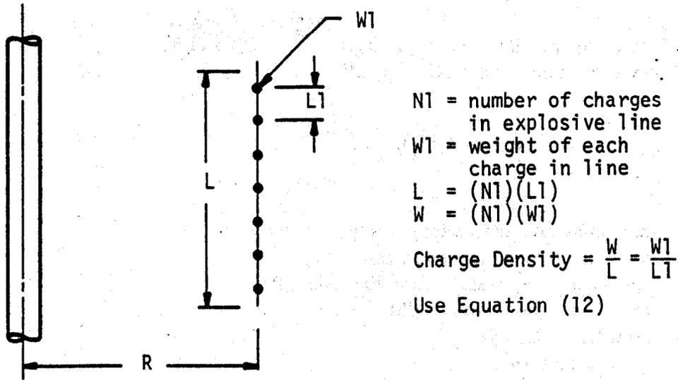
(a) Explosive Line Parallel to Pipeline for  $R \leq L$
