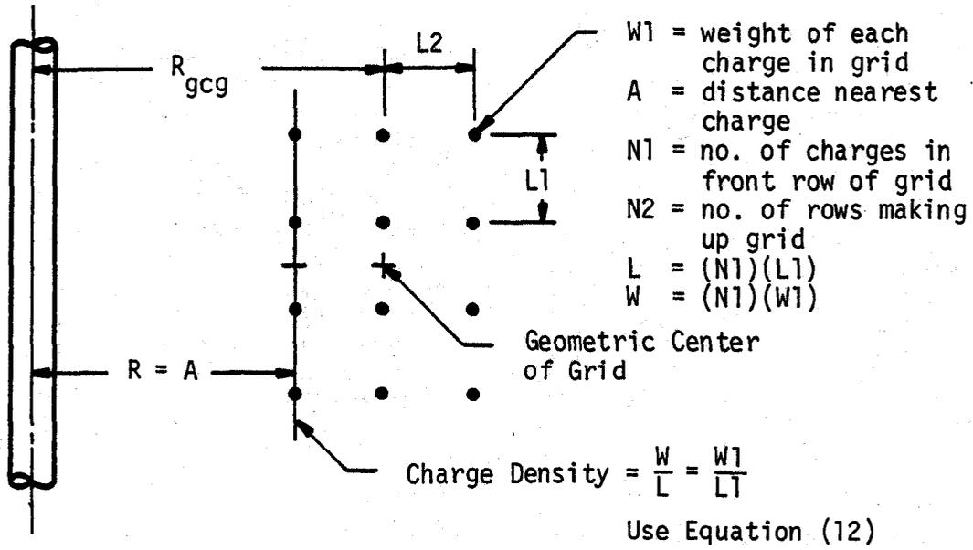
(a) Parallel Grid as Equivalent Parallel Line for  $R < 1.5 L$
