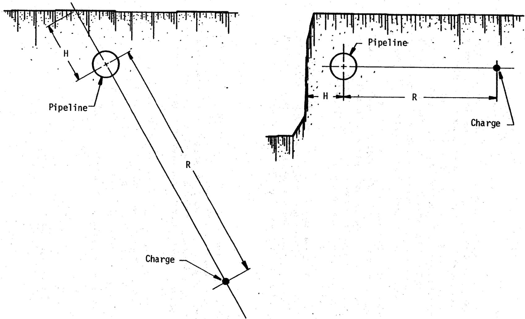
Figure 5. Examples of a Pipeline Near a Free Surface
